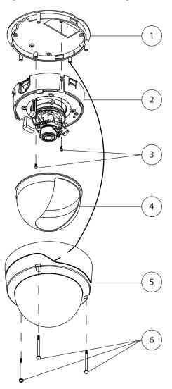
Figure 2-7 Disassembling the 2630 IP Dome Components
